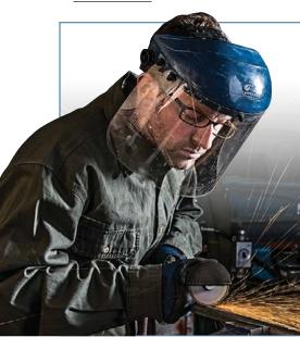
The Norton small diameter cut-off wheel line consists of Type 01/41 straight and Type 27/42 depressed center cut-off wheels from 1-1/2" to 9" diameters. These wheels come in ultra  $\dot{\text{thin}}$  .035" for quick burn-free and burr-free cutting to .125" for more durable applications. All are reinforced for the demanding nature of portable cut-off.
