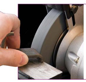
The Norton bench and pedestal wheel line consists of numerous wheel diameters and arbor sizes, abrasive types and grit sizes. Our offering answers all metal removal, deburring, shaping and sharpening needs: white aluminum oxide for high-speed tool steels, brown aluminum oxide for carbon steel, and silicon carbide for non-ferrous metals and carbide tooling.
