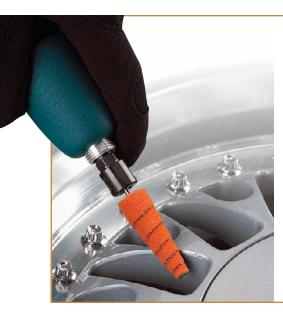
Spiral rolls are strips of abrasive cloth rolled and glued to form a solid shape that is designed to break down during use and reveal the next layer of abrasive.
