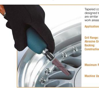
Tapered cone points are strips of abrasive cloth rolled and glued to form a solid shape that is designed to break down during use and reveal the next layer of abrasive. Tapered cone points are similar to cartridge rolls but their shape lends greater accessibility to many difficult-to-reach work areas. They are used for deburring holes and in close tolerance work areas.
