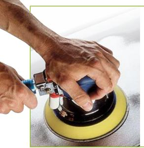
For use on dual action and random orbital sanders. The industry's highest performing and broadest selection of paper discs in PSA (pressure sensitive adhesive) disc rolls and individual discs, and hook and loop discs.
