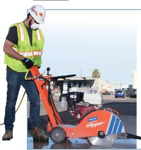
These powerful, self-propelled machines are designed to cut concrete slabs and asphalt and are normally fitted with diamond blades. For inexperienced operators or small jobs, the machines can accommodate these low initial cost, conventional abrasives wheels.
