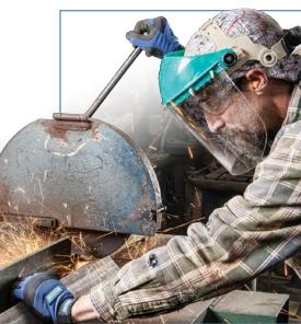
A chop saw is a light, low-horsepower portable machine. Although very similar to a compound miter saw, it is designed for cutting denser materials, like metal bar, tubing or pipe. Chop saw cut-off wheels are designed specifically for this machine with finer grit, softer grades, and reinforcement layers that match the application.
