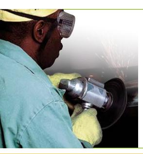
Norton PSA (pressure sensitive adhesive) individual cloth discs are used on four different types of machines and the application changes depending on which machine they are used on.
